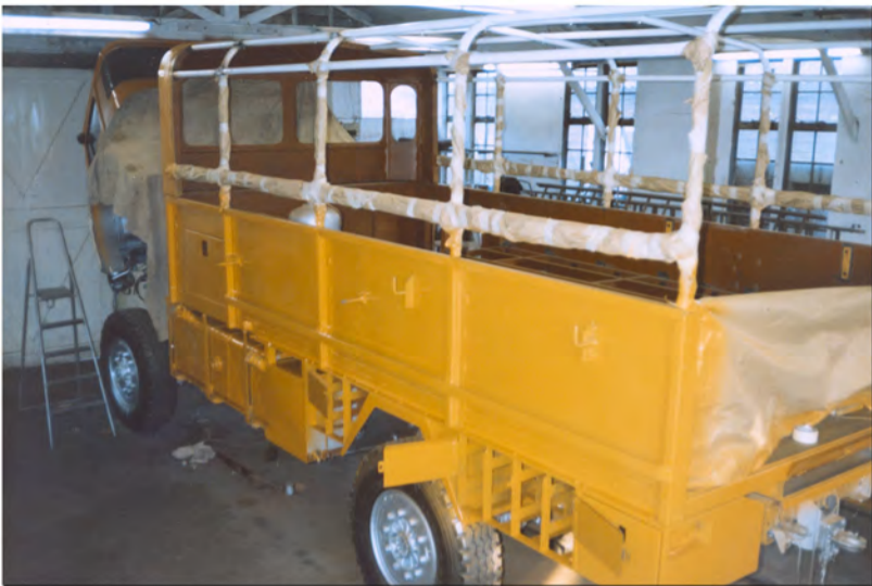
Primary fuel tank, water tank, jerry-can and tool lockers in place.
