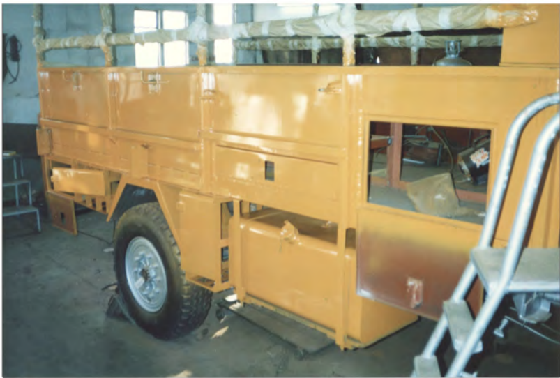
Locker doors giving access to gas cooker and cooking gear in place. Secondary fuel tank, gas bottle, jerry-can and tool lockers in place. Final coat of paint.
