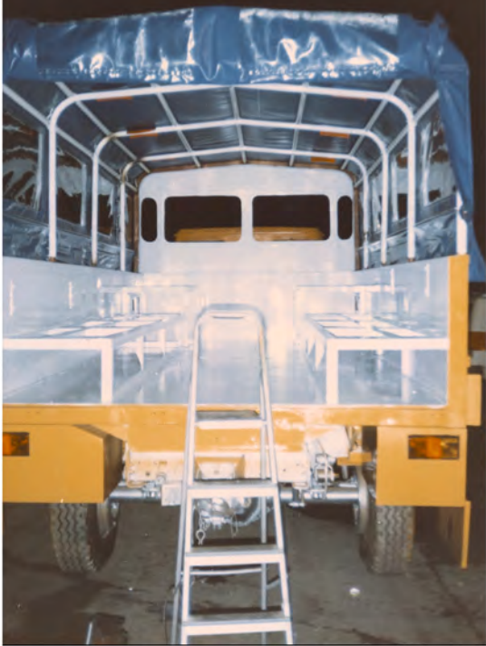
Passenger compartment painted before installing seats and timber lining on seat supports. Tilt fitted over support bars.
