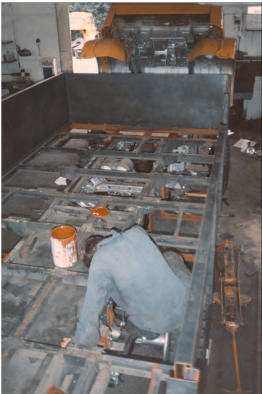
Body installed onto chassis and secured.
