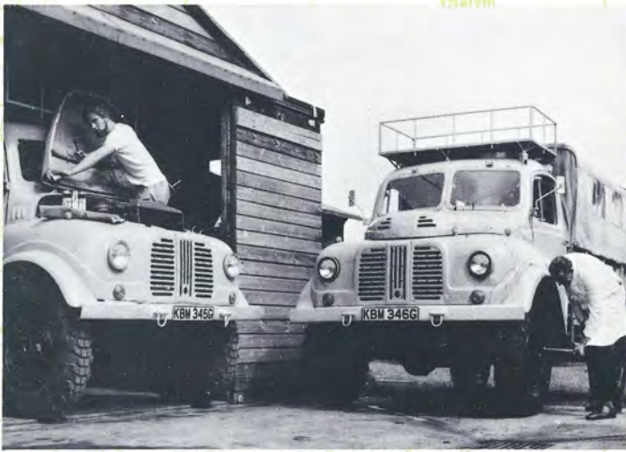
Left. Toni Weldon, expedition leader with Encounter Overland fits a new headlamp unit to a 30cwt. Austin K.9 shod with 'Duramold' pattern 'L' remoulds.
